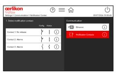
To ensure safe operation for the user, the V-flow Control Unit needs to be connected to the IMM. The available contacts can be adjusted according to specific requirements.
